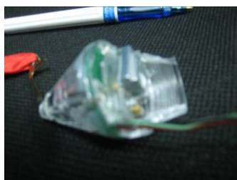
Top and above, safe / arming devices for the MAT 120 cluster munition. © Amnesty International
